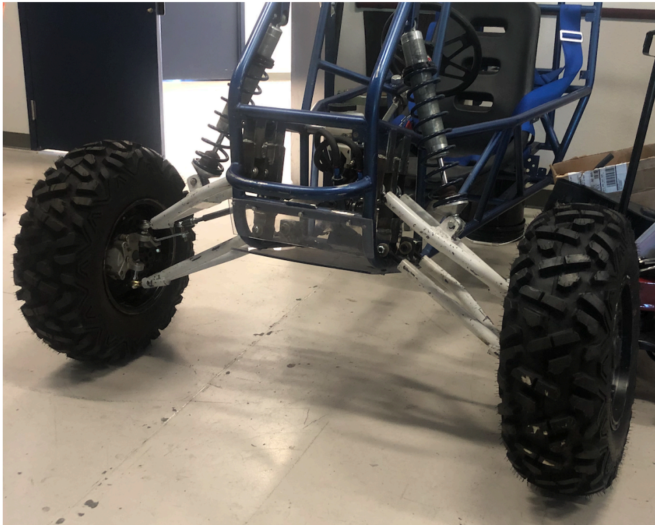
Figure 2: Realigned front suspension
