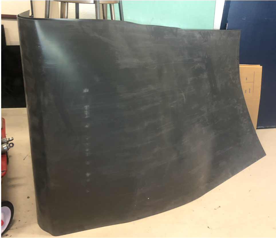
Figure 4: 8 x 4' UL94 Plastic for Firewall
