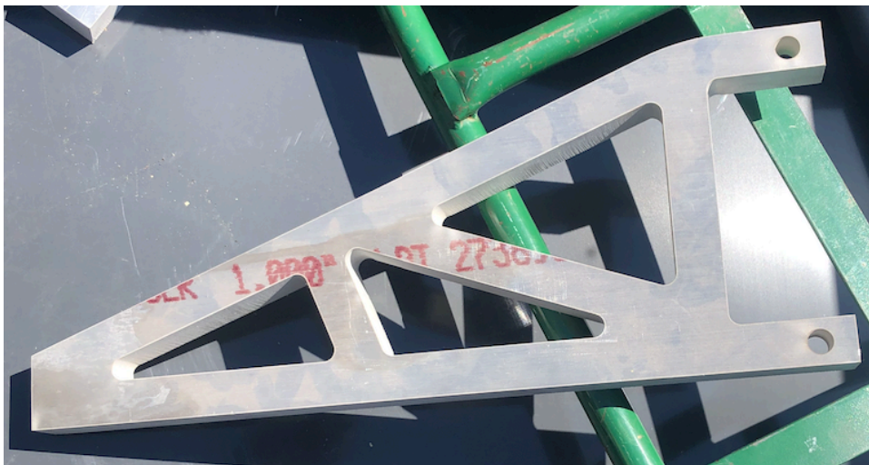
Figure 3: Manufactured trailing arm at MarZee Waterjet Services
